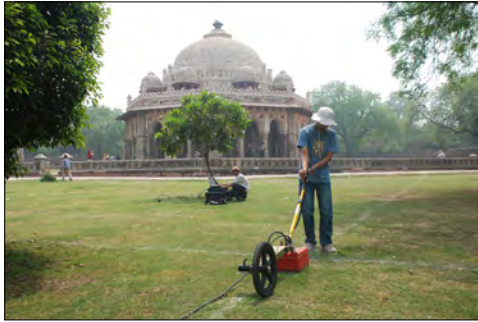
Ground Penetrating Radar Survey
